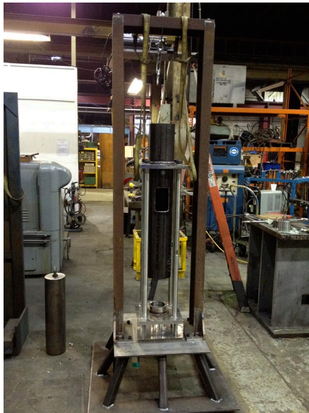
Fig. 5. Single-bubble shockwave fusion system according to Smorodov. In this design 200 lb weight impacts piston that is in contact with glycerin to generate a 1,000 bar shock. A 5-mm deuterium bubble is injected into glycerin prior to impact. The shockwave collapses the bubble launching a spherical converging shock within the bubble's gas, which leads to fusion.
